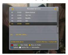
Select the File List menu or alternatively press the 📵 button to display the recorded programme list. The file information is comprised of the following elements: file number, file name, recording time, playing duration, file size and so on.
